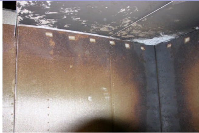
Figure 12. LHS wall panels with skin removed showing char depth on panels 4, 5 and 6.
