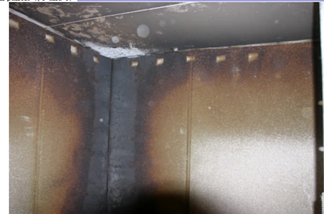
Figure 13. Rear wall panels with skin removed showing char depth on panels 1, 2 and 3.
