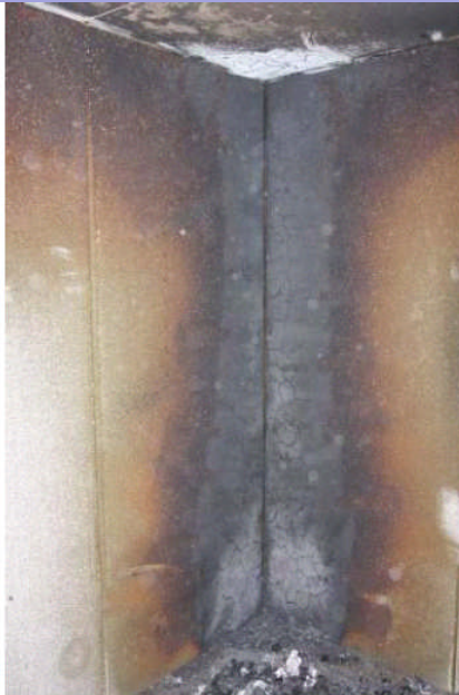
Figure 11. With skin removed charring of foam in region of direct flame contact
